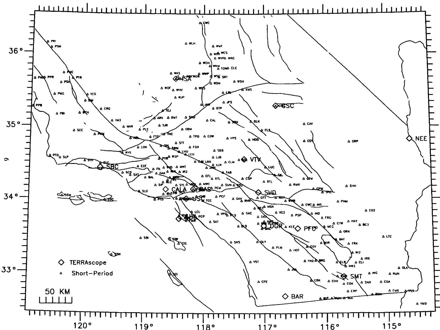
**Figure 1.** Southern California Seismic Network and TERRAscope. Map of all stations operated and maintained by the Pasadena Field Office as well as several stations operated by other agencies that are also digitally recorded, and TERRAscope stations.
